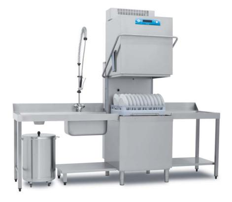
Both River hood dishwashers can be equipped with the NRG heat recovery/steam condensation system. At the end of rinsing, the steam in the wash chamber is extracted and routed to a heat exchanger where it condenses and gives up its heat to the intake water.
